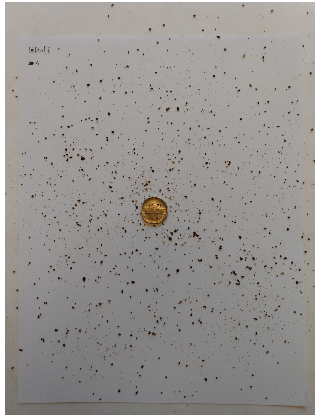
Figure 2: Coffee spread on paper. This image is analyzed in the coffeegrindsize application.
